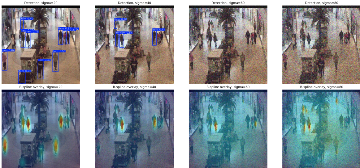
Figure 2. Detection outputs and B-spline heatmap overlays of the clean-pretrained student model under different Gaussian noise levels. The top row shows predicted bounding boxes, and the bottom row shows the corresponding B-spline heatmap overlay.
